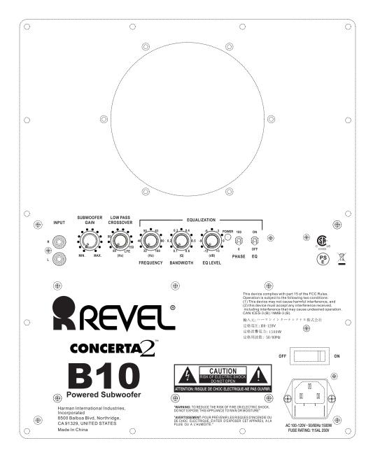
Figure 14: Rear-panel controls and connectors
